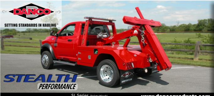
Self-Loader Wrecker: SL-W Series (Worm Gear Winch)
